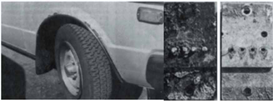
Picture 2: Example of Galvanic Corrosion ( Zehra, Mobin, & Aslam, 2022)
