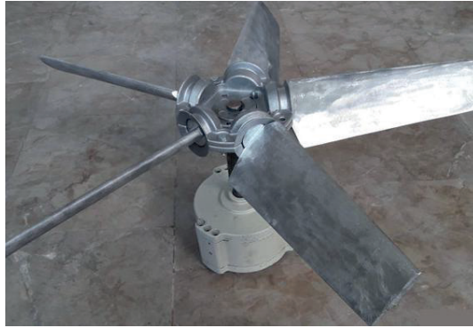
Figure 3.4. Solar chimney turbine blades mounted on the rotor (Ünal, 2019)
