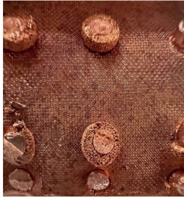
Figure 1. Representative internal structure of a vapor chamber (Oztop et al., 2025).
