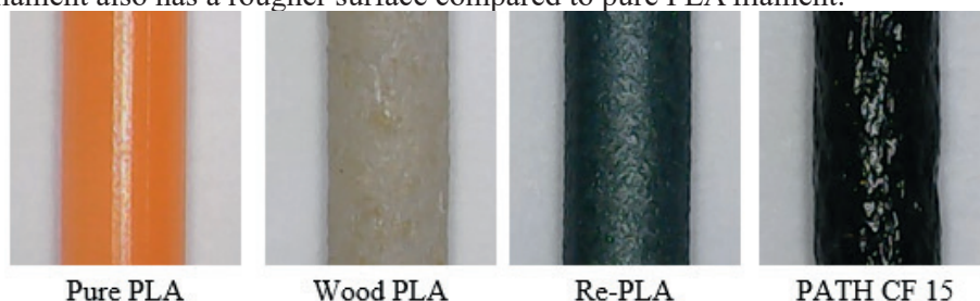
Figure 5. Microscopic images of different filaments.
