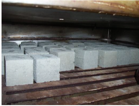
Figure 5. Samples with aggregate from tuff used for high temperature testing.
