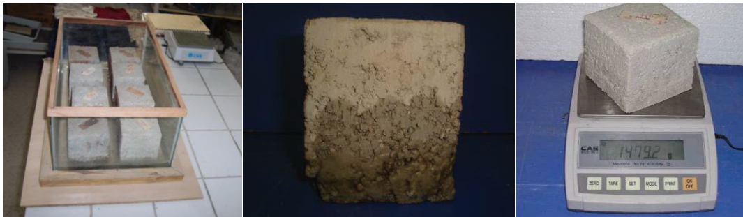
Figure 4. The steps for conducting the capillarity experiment.
