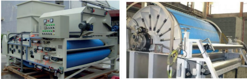
Figure 3. An image of the filter a-drum vacuum filter, b- the belt filter press
