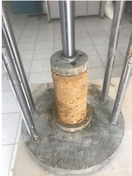
Figure 4. Trimming the size of the sample
