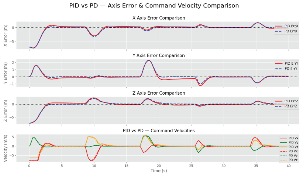
Figure 3 Short impact duration and long recovery time results ( K_p:2 , K_i:0.2 , K_d:0.8 , Force: 0.5N, Interval: 10s)
