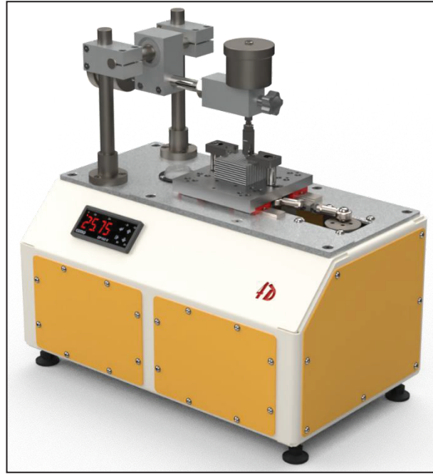
Figure 1. Experimental setup and schematic representation of the reciprocating wear test configuration.
