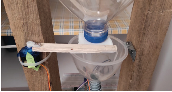
Figure 5. Feed Tank Drain Cover
