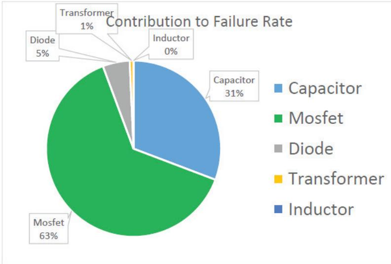
**Fig.5.** *Component Contributions to the Failure Rate*
