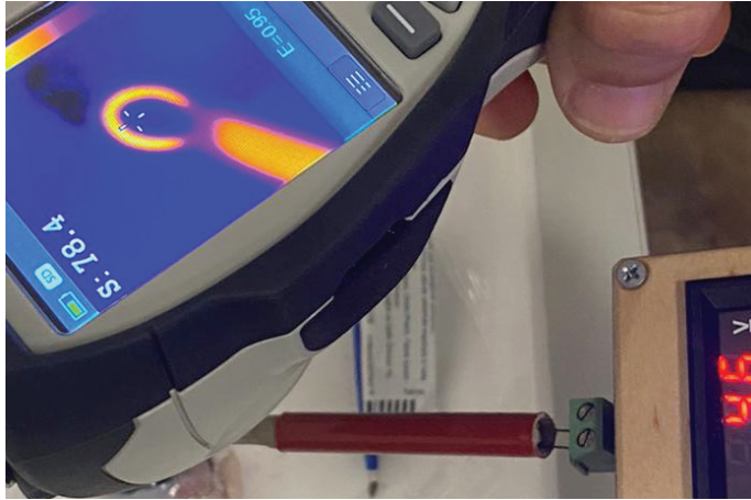
Figure 4. Temperature measurement using Santech ST-980 Thermal Camera
