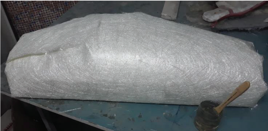
Figure 3.3. Mould wrapped with glass fibre and glass fibre ready for polyester impregnation (Ardıç, 2019)
