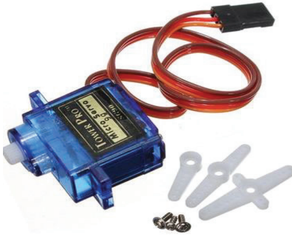
Figure 9. Tower Pro SG90 servo drive.
