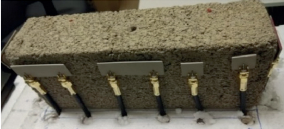
Figure 6. An example of the MI system for non-destructive cracks detection (Jiya et al., 2016)
