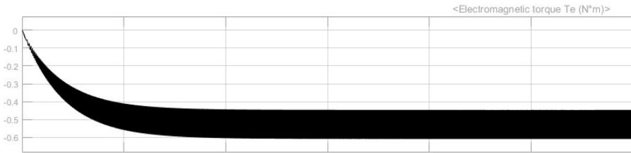
**Figure 16.** Electromagnetic torque generated by the Permanent Magnet Synchronous Generator (PMSG)
