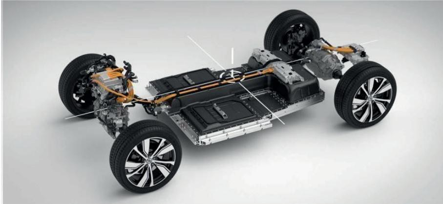
**Figure -1** Electric Vehicle Chassis [11]
