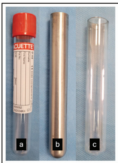
Figure 2. Glass tube (a), titanium tube (b), and nano-titanium-coated tube (c). (Tunalı M, Ercan E, Pat S, Sarıca E, Bağla AG, Aytürk N, Siddıkoğlu D, Bilgin V. Nano-titanium coating on glass surface to improve platelet-rich fibrin (PRF) quality. J Mater Sci Mater Med. 2024 Nov 6;35(1):67)
