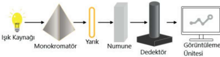
Figure 4.5. General working principle of a spectrophotometer.
