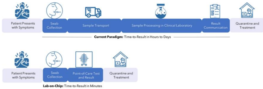
Figure 2. How might a LoC diagnosis impact a patient's workflow? Current classic diagnostic workflows include collecting samples, transporting them, processing them, and delivering the results to the patient. (Bottom) LOC technologies enable on-chip POC tests with results in minutes (Carly Tymm et al., 2020).
