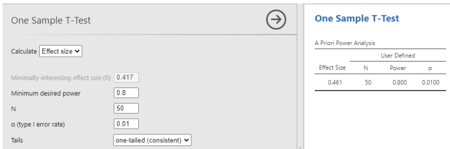
Figure 10. Calculating effect size with values defined in a one-tailed hypothesis test in jpower
