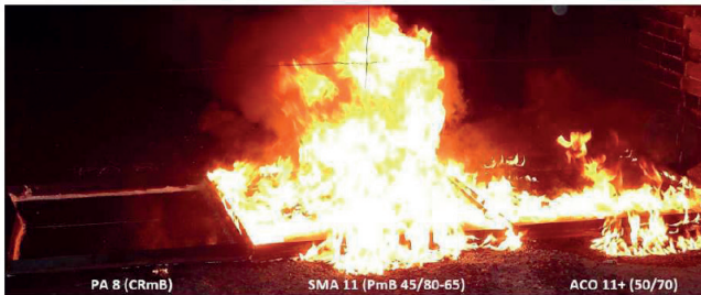
Figure 4. The comparison of the gasoline combustion of the surface of different asphalt mixtures: porous mixture (PA 8), stone mastic asphalt (SMA11, with ~7% of bitumen) and typical asphalt concrete (ACO 11) (Fiedler et al., 2018)
