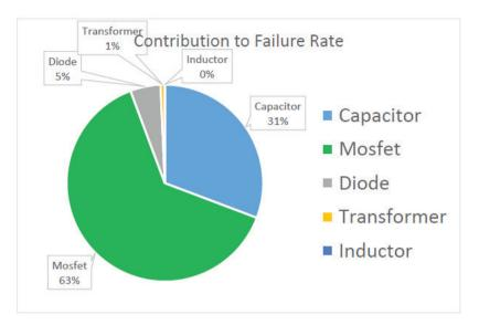
Fig.5. Component Contributions to the Failure Rate
