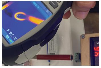
Figure 4. Temperature measurement using Santech ST-980 Thermal Camera
