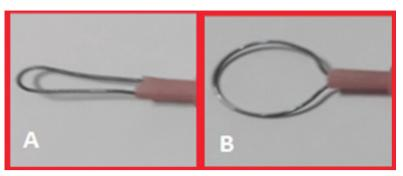
Figure 2. The SMA (A: Before heated, B: After heated)
