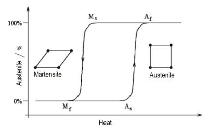
Figure 1. Temperature Changes and Hysteresis Curve of SMA[19,20]
