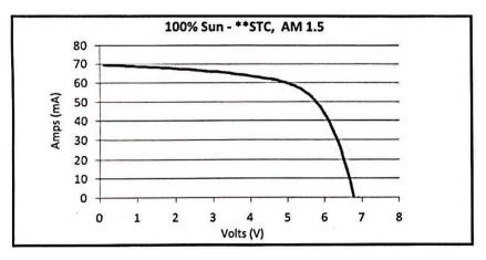
Fig. 2. Current-Voltage graph of the test sample
