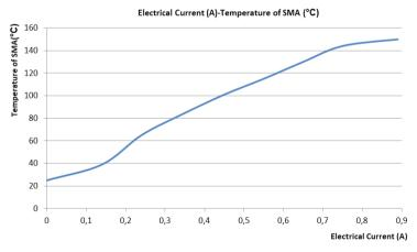
Figure 5. Graphic of the relation of electrical current - temperature of SMA
