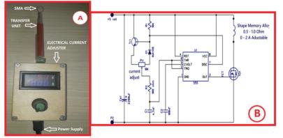
Figure 3. SMAC and electronic circuit diagram.
