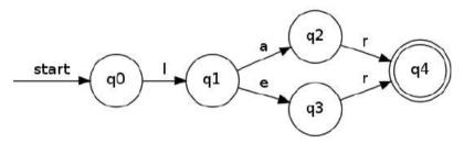
Figure 4. The automaton for the plural morpheme
