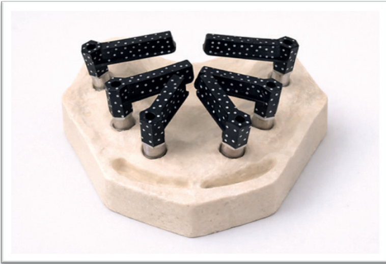
Figure 5: The intraoral photogrammetry system Aoralscan Elite is illustrated.
