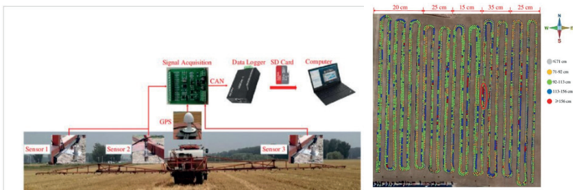
Figure 2. Sprayer boom height detection system architecture and Distribution map of boom height variation in a wheat stubble field (Dou et al., 2021).
